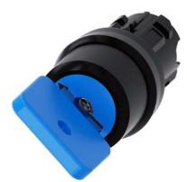
Key-operated switch O.M.R, 22 mm, round, plastic, lock number 73038, blue, with 2 keys, 2 switch positions O-I, latching, actuating angle 90°, 10:30h/13:30h, key removal O+I, with laser labeling, upper case
