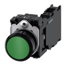
Pushbutton, 22 mm, round, plastic, green, pushbutton, flat, momentary contact type, with holder 1 NO+1 NC, spring-type terminal, Z=20-unit packaging
