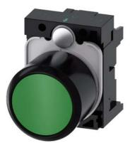
Pushbutton, compact, with extended stroke (12 mm), 22 mm, round, plastic, green, pushbutton, flat, momentary contact type, with holder, with laser labeling, symbol number according to, ISO 7000 or IEC 60417
