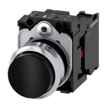
Pushbutton, 22 mm, round, metal, shiny, black, pushbutton, raised, momentary contact type, with holder, 1 NC, screw terminal, with laser labeling, symbol number according to, ISO 7000 or IEC 60417
