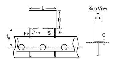
Series Dielectric Metallized Polypropylene Style Radial Features MKP EMI Safety RoHS Lead Wire Leads Safety Class X1 Qualifications ENEC, UL, cUL, CQC AEC-Q200 No THB Performance No Component Weight 3.177 g Miscellaneous ClimCat: 40/110/56/B Shelf Life 104 Weeks
