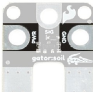
Power connection pads.
