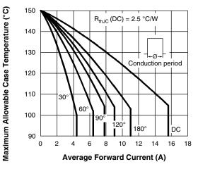
Fig. 2 - Current Rating Characteristics
