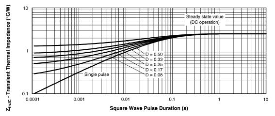
Fig. 8 - Thermal Impedance  $Z_{\text{thJC}}$  Characteristics
