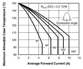
Fig. 1 - Current Rating Characteristics
