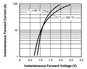
Fig. 7 - Forward Voltage Drop Characteristics
