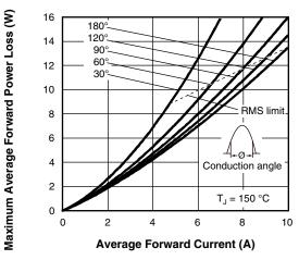
Fig. 3 - Forward Power Loss Characteristics
