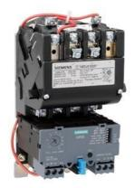
Non-reversing motor starter Size 1 Single phase full voltage Solid-state overload relay OLRelay amp range 5.5-22A 190-220/220-240V 50/60HZ coil Combination type No enclosure
