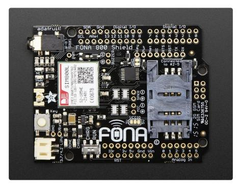
This shield fits on top of any classic Arduino or compatible, and packs a surprising amount of technology into it's little frame. At the heart is a GSM cellular module (we
