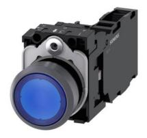
Illuminated pushbutton, 22 mm, round, plastic with metal front ring, blue, pushbutton, flat, momentary contact type, with holder, 1 NO+1 NC, LED module with integrated LED 24 V AC/DC, screw terminal
