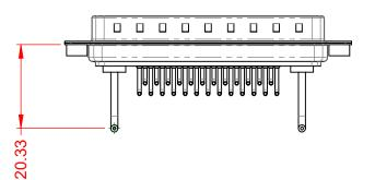
10A (CURRENT) **POWER/CO-AX CONTACT RATING:** (IF PRESENT) SIGNAL CONTACT CURRENT RATING: 5A PER CONTACT SIGNAL CONTACT RESISTANCE:  $10m\Omega$  MAX. **INSULATOR RESISTANCE:** 5000MΩ min. DIELECTRIC
