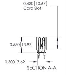
717 Series Ultra-Mate Card Edge Connector - Press Fit Part Number: 717-034-560-201 **EDAC INC** THESE DRAWINGS AND SPECIFICATIONS ARE THE PROPERTY OF EDAC INC.,AND TORONTO, ONTARIO
