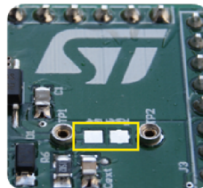
Figure 5. Pads for soldering SMD resistor
