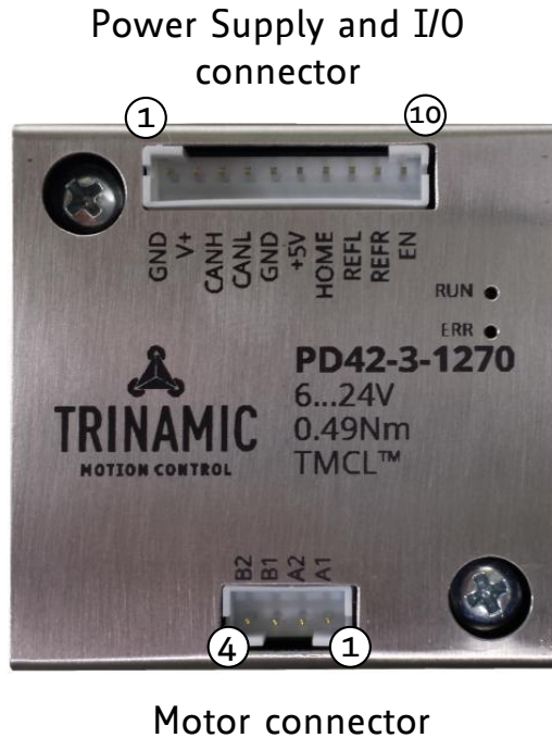
Figure 8: TMCM-1270 connectors
