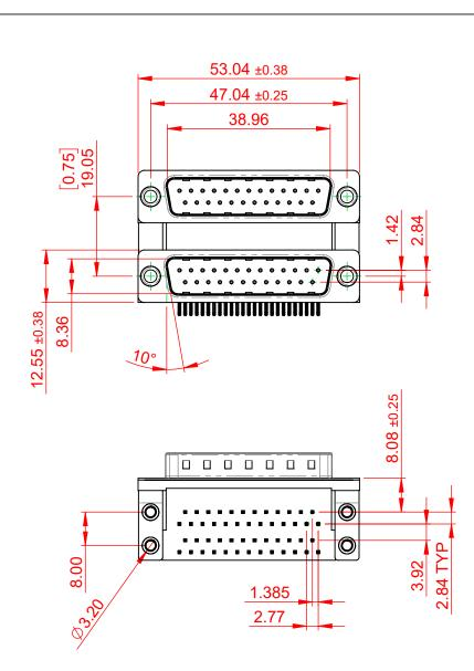
THIS IS A C.A.D. GENERATED DRAWING TOLERANCE UNLESS OTHERWISE SPECIFIED DO NOT MAKE MANUAL REVISIONS TO MASTER. .X ±0.25 .XX ±0.13
