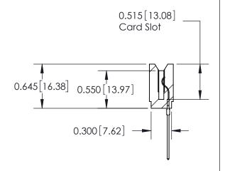
ACAD REFERENCE NO. 737 Series Ultra-Mate Card Edge Connector - Press Fit DRAWN: Part Number: 737-014-541-106 CHECKED: **EDAC INC** SCALE: THESE DRAWINGS AND SPECIFICATIONS ARE THE PROPERTY OF EDAC INC.,AND TORONTO, ONTARIO SHALL NOT BE REPRODUCED, OR COPIED DRAWING NUMBER CANADA OR USED AS THE BASIS FOR THE MANUFACTURE OR SALE OF APPARATUS YOUR CONNECTION TO QUALITY & SERVICE WITHOUT WRITTEN PERMISSION.
