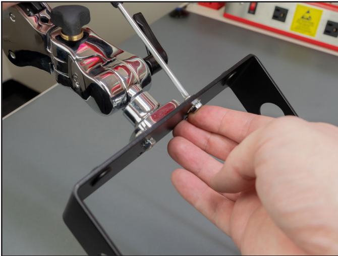
Figure 5. Securing the boom arm to 963E Benchtop Air Ionizer's metal bracket
