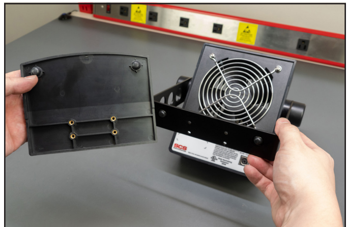
Figure 3. Removing the plastic base plate from the 963E Benchtop Air Ionizer
