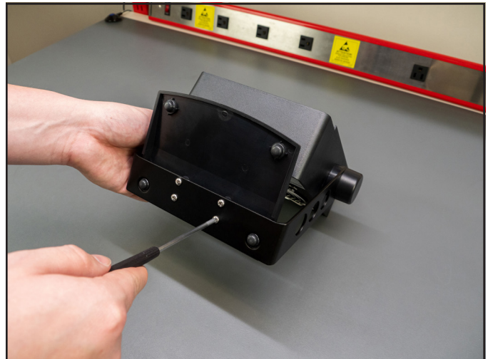
Figure 2. Removing the 4 screws underneath the 963E Benchtop Air Ionizer
