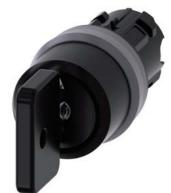
Key-operated switch O.M.R, 22 mm, round, plastic with metal front ring, lock number 73034, black, with 2 keys, 3 switch positions I-O<II, left latching, right momentary contact type, actuating angle 2x45°, 10:30h/12h/13:30h, Key removal I Z=50-unit packaging
