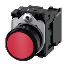
Pushbutton, 22 mm, round, plastic, red, pushbutton, flat, momentary contact type, with holder 1 NO, screw terminal, with laser labeling, upper case and lower case, always upper case at the beginning of the word
