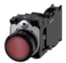
Illuminated pushbutton, 22 mm, round, plastic, red, pushbutton, flat, momentary contact type, with holder, 1 NO+1 NC, LED module with integrated LED 110 V AC, spring-type terminal, with laser labeling, lower case
