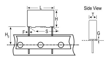
General Information Series F872 Dielectric Metallized Polypropylene Style Radial Features MKP EMI Safety RoHS Yes Lead Wire Leads Safety Class X1 Qualifications ENEC, UL, cUL, CQC AEC-Q200 No THB Performance No Component Weight 5.624 g Miscellaneous ClimCat: 40/110/56/B Shelf Life 104 Weeks
