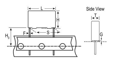
Series F881 Dielectric Metallized Polypropylene Style Radial Features MKP EMI Safety RoHS Lead Wire Leads Safety Class Qualifications ENEC, UL, cUL, CQC AEC-Q200 No THB Performance No 4.858 g Component Weight Miscellaneous ClimCat: 40/110/56/B Shelf Life 104 Weeks
