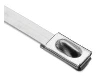
316 grade stainless steel offers excellent resistance to salt spray, corrosion, weather and chemical resistance.Self locking, ball bearing mechanism for quick and easy installation, either by hand or by tensioning tool.
