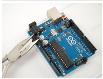
Attach the Arduino securely by screwing on the last two hex nuts
