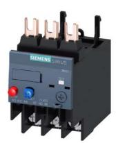
Overload relay 27...32 A Thermal For motor protection Size S0, Class 10 Contactor mounting Main circuit: Ring cable lug Auxiliary circuit: ring cable lug Manual-Automatic-Reset
