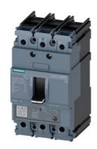
circuit breaker 3VA5 UL frame 125 breaking capacity class M 35kA @ 480 V 3-pole, line protection TM230, FTAM, In=50A overload protection Ir=50A fixed short-circuit protection Ii=5...10 x In UL489 SB (naval), 50 deg. cel. nut keeper kit on both sides
