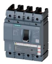
circuit breaker 3VA5 UL frame 250 breaking capacity class H 65kA @ 480V 4-pole, line protection TM230, FTAM, In=200A overload protection Ir=200A fixed short-circuit protection li=5...10 x In N conductor protection 100% without connection
