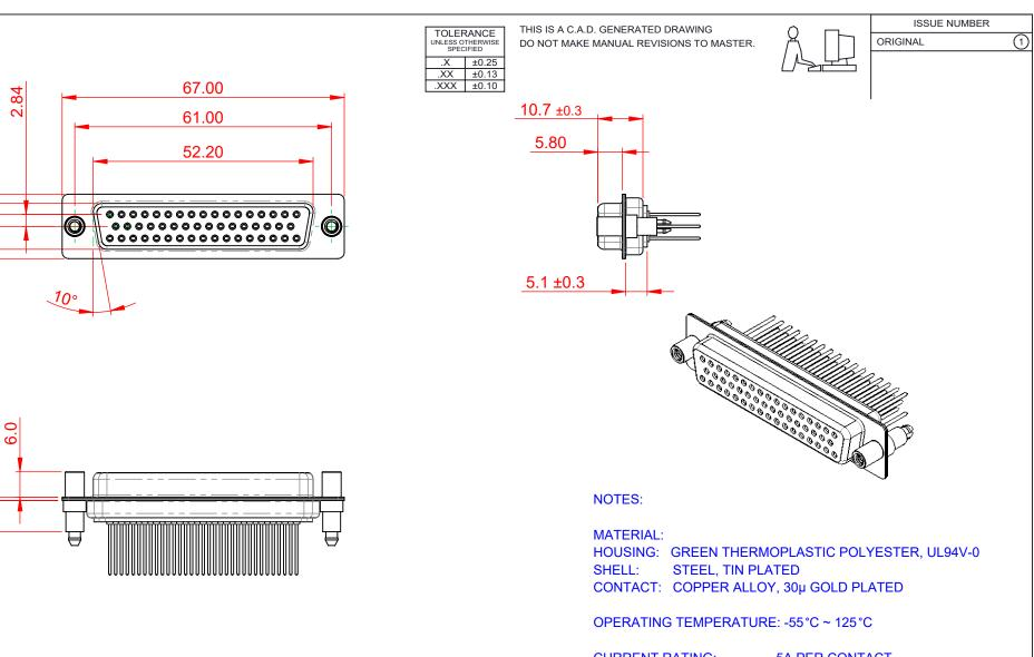
**CURRENT RATING: 5A PER CONTACT** CONTACT RESISTANCE:  $25m\Omega$  MAX. INSULATOR RESISTANCE: 5000MΩ min. DIELECTRIC WITHSTANDING VOLTAGE: 1000V AC rms
