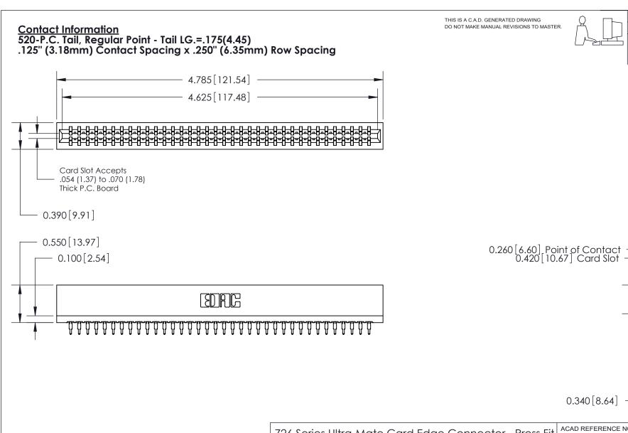
ACAD REFERENCE NO. 726-ENG MASTER 726 Series Ultra-Mate Card Edge Connector - Press Fit DRAWN: J.LEE DATE: AUG 20/09 Part Number: 726-072-520-201 CHECKED: DATE: **EDAC INC** SCALE: SHEET 1 OF 2 THESE DRAWINGS AND SPECIFICATIONS ARE THE PROPERTY OF EDAC INC.,AND TORONTO, ONTARIO SHALL NOT BE REPRODUCED, OR COPIED DRAWING NUMBER **ISSUE** CANADA OR USED AS THE BASIS FOR THE 726-ENG MASTER MANUFACTURE OR SALE OF APPARATUS YOUR CONNECTION TO QUALITY & SERVICE WITHOUT WRITTEN PERMISSION.
