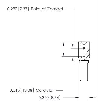
ACAD REFERENCE NO. 746-ENG MASTER 746 Series Ultra-Mate Card Edge Connector - Press Fit DRAWN: J.LEE DATE: AUG 20/09 Part Number: 746-034-553-201 CHECKED: DATE: **EDAC INC** SCALE: SHEET 1 OF 1 THESE DRAWINGS AND SPECIFICATIONS ARE THE PROPERTY OF EDAC INC.,AND TORONTO, ONTARIO SHALL NOT BE REPRODUCED, OR COPIED DRAWING NUMBER CANADA OR USED AS THE BASIS FOR THE 746-ENG MASTER MANUFACTURE OR SALE OF APPARATUS YOUR CONNECTION TO QUALITY & SERVICE WITHOUT WRITTEN PERMISSION.
