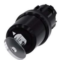
key-operated switch Siemens, 22 mm, round, plastic, special lock, with 2 keys, 2 switch positions O-I, latching, actuating angle 90°, 10:30h/13:30h, key removal O
