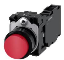
Pushbutton, 22 mm, round, plastic, red, pushbutton, raised, momentary contact type, with holder 1 NO+1 NC, screw terminal, with laser labeling, symbol number according to, ISO 7000 or IEC 60417
