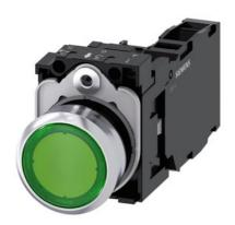
Illuminated pushbutton, 22 mm, round, Metal, shiny, green, pushbutton, flat, momentary contact type, with holder, 1 NO+1 NC, LED module with integrated LED 230 V AC, screw terminal, with laser labeling, upper case and lower case, always upper case at beginning of line
