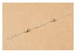
These have been twisted together and then soldered for extra strength.
