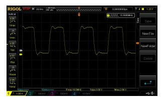
You may notice a bit of over shooting in the picture above and a bit of ringing in the signal. There are a number of reasons why this is happening. I'm terminating my signal on a  $1M\Omega$  oscilloscope probe, when I should be using a  $50\Omega$  instead. I also have an extended ground cable on the probe, which should be shortened for better signal capture. None the less, I hope that this is still demonstrative of the SparkFun Clock Generator capabilities.
