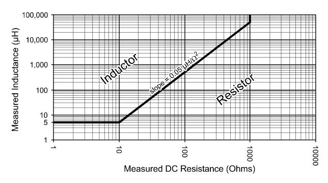
For example, if the inductance of your component is measured at  $100\mu H$  and it has a DC resistance of  $100\Omega$ , then the LCR40 will tell you that you have a resistor. If however the resistance was only  $10\Omega$ , then the LCR40 will tell you that you have an inductor.
