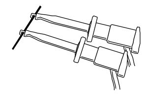
Before you start the compensation procedure, attach a small length of tinned copper wire between the two test probes. Now let the leads rest on a non-conductive surface, try not to touch them during the compensation procedure.
