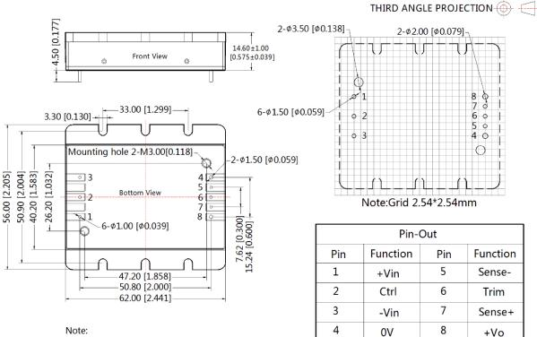
Note: Unit: mm[inch] Pin1, 2, 3, 5, 6, 7's diameter: 1.00[0.039]Pin4, 8's diameter: 1.50[0.059]Pin diameter tolerances:  $\pm 0.10[\pm 0.004]$ General tolerances:  $\pm 0.50[\pm 0.020]$ Mounting hole screwing torque: Max 0.4 N·m
