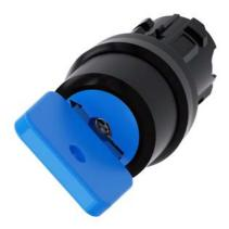
Key-operated switch O.M.R, 22 mm, round, plastic, lock number 73038, blue, with 2 keys, 2 switch positions O<I, momentary contact type, Actuating angle 45°, 10:30h/12h, key removal O, with laser labeling, inscription or symbol Customer-specific selection with SIRIUS ACT configurator (CIN)
