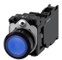
Illuminated pushbutton, 22 mm, round, plastic, blue, pushbutton, flat, momentary contact type, with holder, 1 NO+1 NC, LED module with integrated LED 24 V AC/DC, spring-type terminal, with laser labeling, upper case and lower case, always upper case at beginning of line
