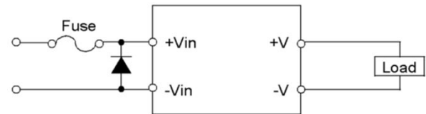
Fig.1-5 Protection for Reversed Input Connection
