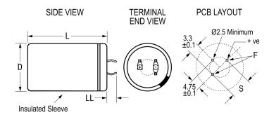
**General Information** Series PEH536 Dielectric Aluminum Electrolytic Description Snap-In, Aluminum Electrolytic RoHS Yes Lead 3 Pin Short AEC-Q200 No **Component Weight** 39 g Notes Add 0.5mm To D And 1mm To L For Sleeving. Shelf Life 208 Weeks
