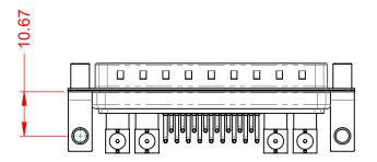
**OPERATING TEMPERATURE:** -55°C ~ 125°C 50Ω (IMPEDANCE) POWER/CO-AX CONTACT RATING: (IF PRESENT) SIGNAL CONTACT CURRENT RATING: 5A PER CONTACT SIGNAL CONTACT RESISTANCE:  $10m\Omega$  MAX. **INSULATOR RESISTANCE:** 5000MΩ min.
