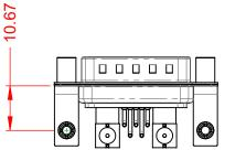
75Ω (IMPEDANCE) POWER/CO-AX CONTACT RATING: (IF PRESENT) SIGNAL CONTACT CURRENT RATING: 5A PER CONTACT SIGNAL CONTACT RESISTANCE:  $10m\Omega$  MAX.
