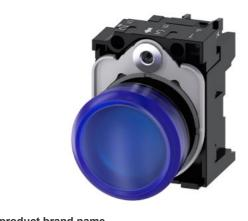
Indicator lights, 22 mm, round, plastic, blue, lens, smooth, with holder, LED module, with integrated LED 24 V AC/DC, screw terminal, with laser labeling, inscription or symbol Customer-specific selection with SIRIUS ACT configurator (CIN)
