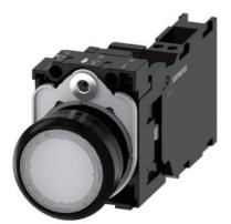
Illuminated pushbutton, 22 mm, round, plastic, white, pushbutton, flat, momentary contact type, with holder, 1 NO+1 NC, LED module with integrated LED 110 V AC, spring-type terminal, with laser labeling, inscription or symbol Customer-specific selection with SIRIUS ACT configurator (CIN)
