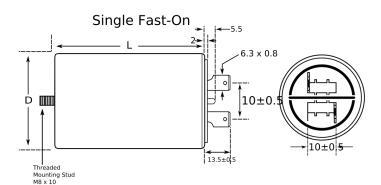
Series C27 Dielectric Film/Foil Polypropylene Style Plastic Case and Cover, Ultra Sonically Welded Description Ultra Sonically Welded Seal, Safety Class PO, Features UL 94 V0 Disk **RoHS** Yes Lead Fast On (1+1) UL, VDE, UL (Construction Only), UL\_94 VO Qualifications Disk AEC-Q200 No Component 26 g Weight
