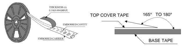
The force for peeling off cover tape is 10 to 70 grams in the arrow direction.
