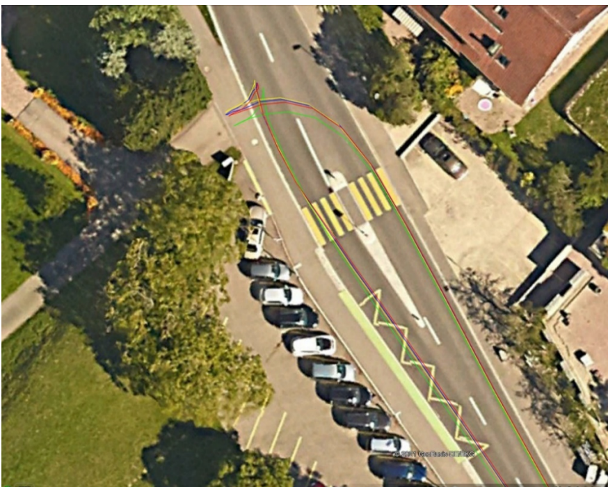
Figure 7: NEO-M8(Q/N) in red, NEO-M8M in blue, NEO-M8J in yellow, and reference position tracks (in green) in rural areas while changing heading of motion
