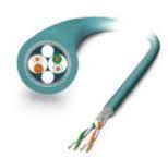
Network cable, Ethernet CAT5 (100 Mbps), 4-position, PUR halogen-free, water blue RAL 5021, shielded, free cable end, on free cable end, cable length: 100 m
