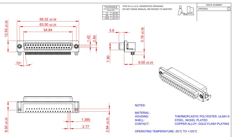
CURRENT RATING: CONTACT RESISTANCE: INSULATOR RESISTANCE: DIELECTRIC
