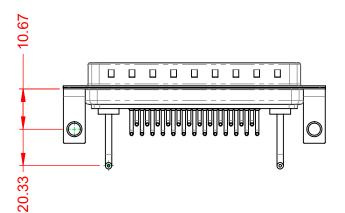
OPERATING TEMPERATURE: $-55^{\circ}C \sim 125^{\circ}C$ POWER/CO-AX CONTACT RATING:10A (CURRENT)(IF PRESENT)SIGNAL CONTACT CURRENT RATING:5A PER CONTACTSIGNAL CONTACT RESISTANCE:10m $\Omega$  MAX.INSULATOR RESISTANCE:5000M $\Omega$  min.DIELECTRICDIELECTRIC
